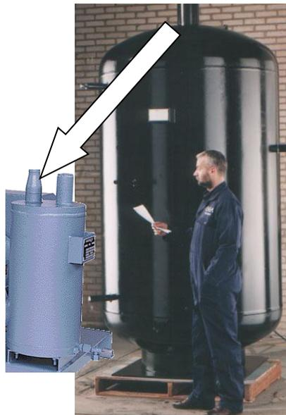
A new type of gascoolers with direct expansion is developed where refrigerant charge could be reduced with 99% and the contracting costs with 75%, both related to the conventional open flash intercooler.
