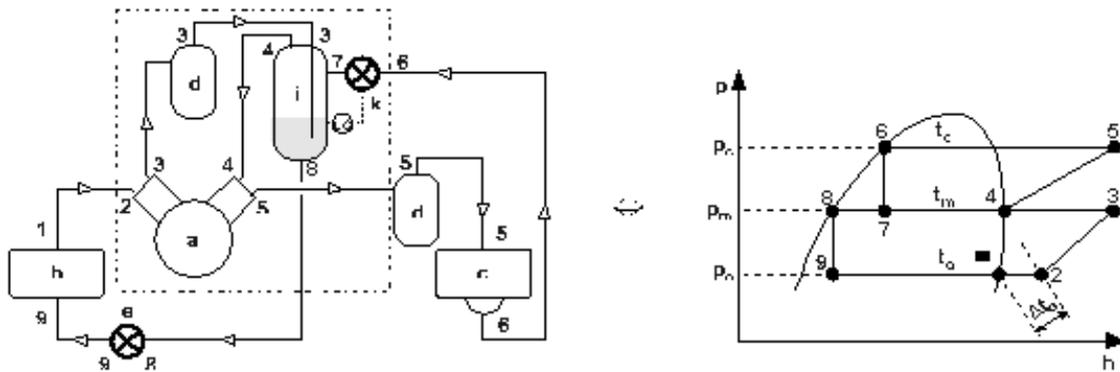
To understand the function of the open flash intercooler, we have to understand the bubble mechanism.
