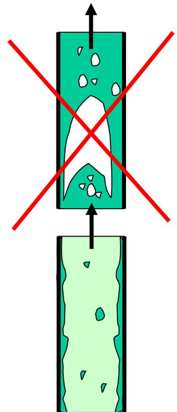
To cool down the first stage superheated discharge gas and to evaporate the injected refrigerant it is a must to create a two-phase ringflow in the annular spacing of the pipe in pipe gascooler.
