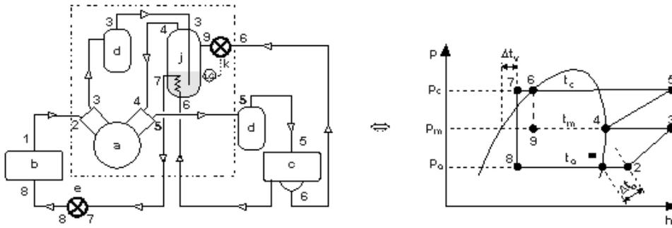
To obtain maximum pressure difference over the injection valves on pumpstations or evaporators, a subcooling coil is submerged in the boiling liquid of the open flash intercooler. The heat transfer calculation is the same as used to select flooded liquid coolers.
