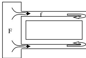
Pressure loss along the annular length =  $\lambda \times L/d_h$ ,  $\lambda$  is dependent of refrigerant, flashgas-amount, mass-flow and annular-geometry.
